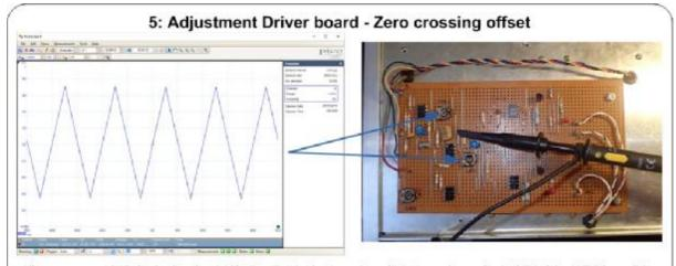
Allow a warm up of 15mins to allow for stabilisation. Set the front panel sensitivity to maximum. Centre VR1. Adjust VR2 for an DC average of 0V (until the saw tooth is centred on the 0V axis).
