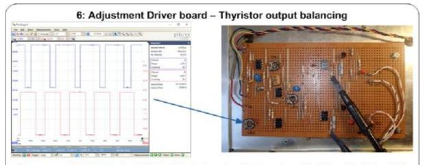
Allow a warm up of 15mins to allow for stabilisation. Set the front panel sensitivity to maximum. Adjust VR3 until the light is as bright as it will go. Then with the sensitivity set minimum rotate the pot anticlockwise until the lamp is fully off
